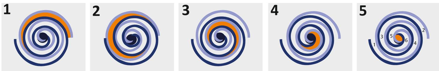
**1** Compression is accomplished by reducing the size of the outside pockets as the scroll relative motion moves them inwards towards the discharge port
